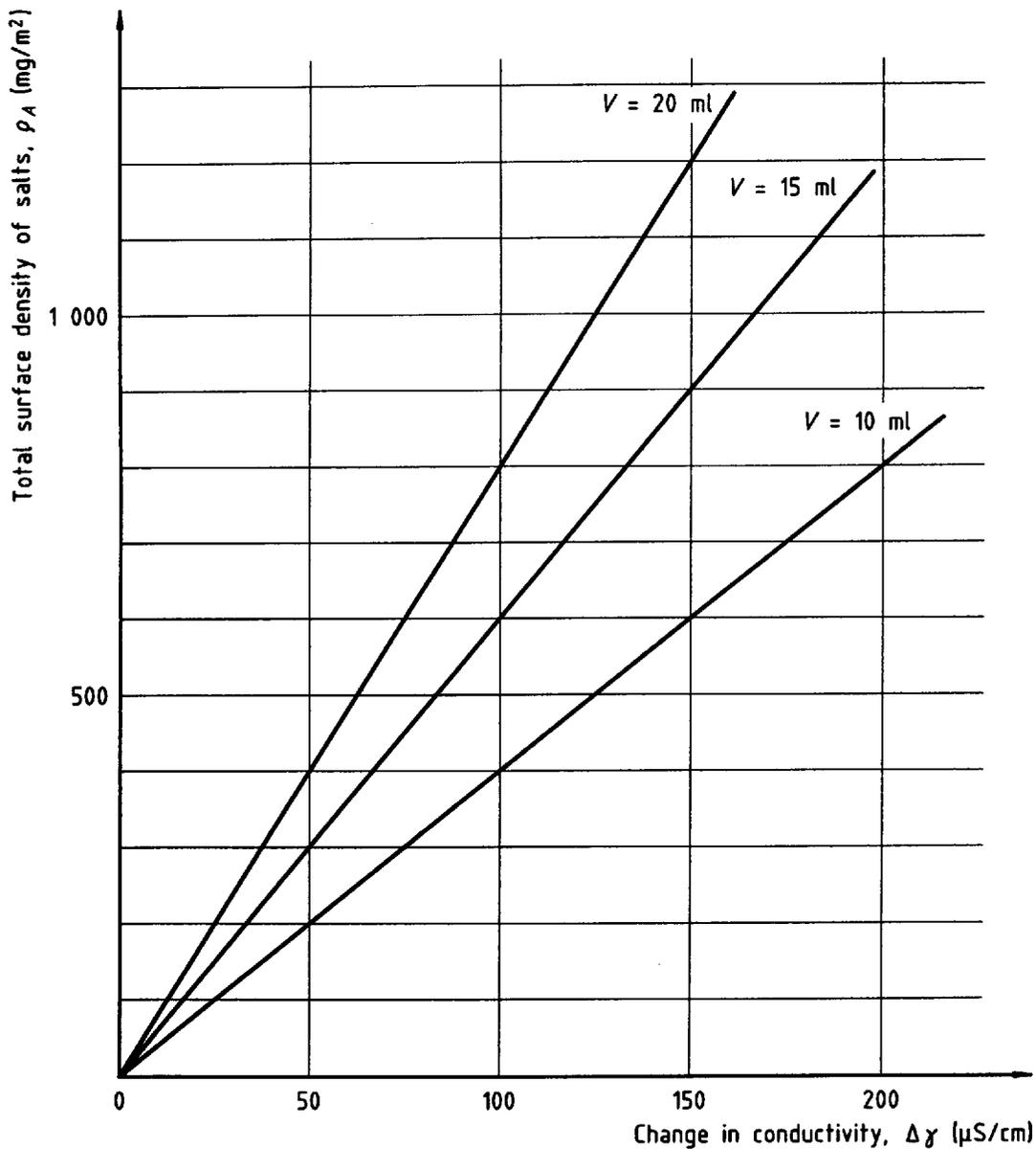
NOTE — Each straight line corresponds to a different volume of water in the beaker. In each case, the patch size is A-1250, in accordance with ISO 8502-6.
